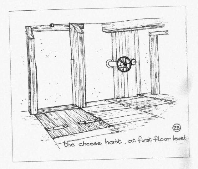
FIGURE 4: Sketch of cheese hoist on first floor, now removed; from report by architect Leach Rhodes and Walker, 1962 The ceiling is of crossbeam type, with deep-chamfered beams approximately one foot in diameter and intermediate joists exposed. In the southeast corner of the room is the upper portion of the kitchen fireplace, with, just above floor level, a stone inscribed:
