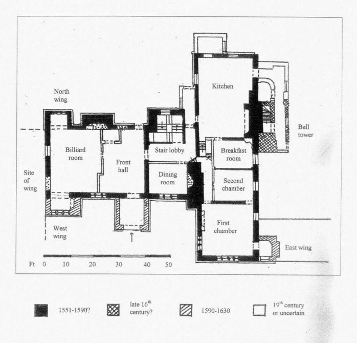
FIGURE 1: Ground floor plan, showing names of rooms and building sequence
