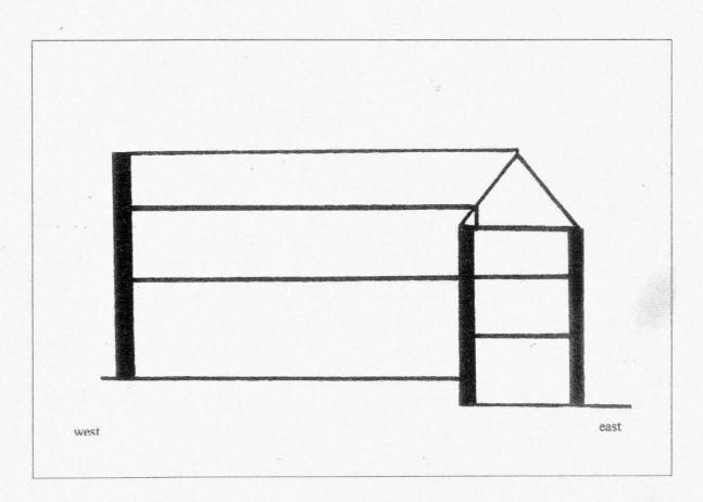
FIGURE 2: Sketch, not to scale, showing floor levels in hall range and wing
